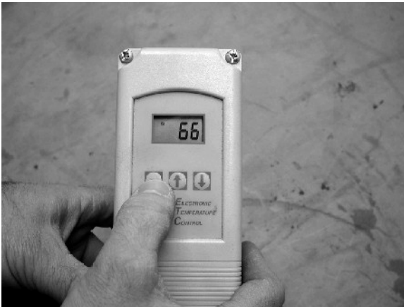
The thermostat shows the current ambient temperature when connected to the Dragon.
